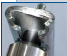
Example for an extended front sleeve with a special nose piece.
