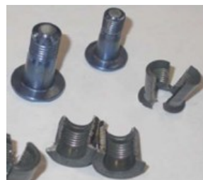
XBF-LV collars cut with Double Blades hydraulic cutter
