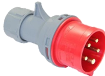
3 x 400 Volts 5 pins plug, 3 phases, neutral and earth connection 16 Amps
