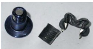
SLFC-MV collars cut with FCMV hydraulic cutter
