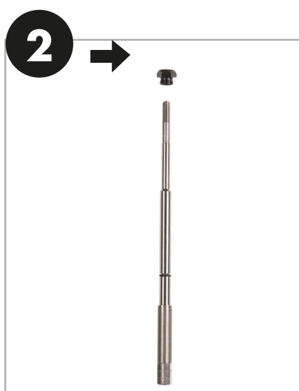
2. Installation Install the threaded mandrel and nosepiece
